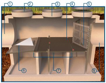
Fig.1 The Hydro DryScreen® has internal components designed to increase particulate pollutant capture and minimize nutrient leaching.
