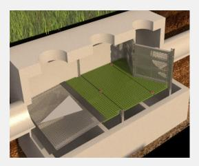
As stormwater enters the Hydro DryScreen® chamber, the flow is diffused and slowed by the Flow Spreader. Gross solids are conveyed around the spreader and captured on the horizontal screen (**Fig.1**). This process enables our screen to go four times longer before blinding compared to other next generation baffle boxes.
