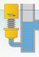
Based on the simple science of buoyancy, Thirsty Duck employs groundbreaking flow control technology that drains water at a nearly constant rate — requiring less detention volume and therefore reducing stormwater system size by up to 50%.
