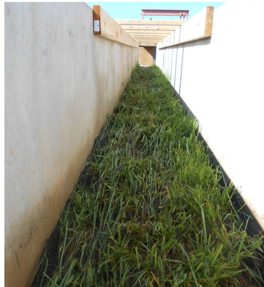
One test plot of the vegetated W3000 HPTRM prior to flow events.
