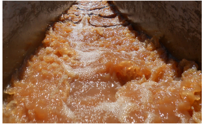
Example of the turbulence created in the flume under test flow conditions
